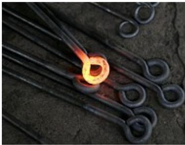
*Convection* is one of the modes of heat transfer here. But, so is *radiation*. Remember, that the iron rod is too hot as compared to the surrounding temperature and so it will radiate a lot of heat. In fact, the heat is so much that the rod glows bright red. (If you know a little about the EM spectrum, you would know that when the emission from a body also includes the visible spectrum, we can actually see (a part of) the emission spectrum.)
