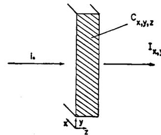
Fig. 1. An intensity image  $I_{x,y}$  as reproduced by the transmission of light through a volume concentration of amorphous silver  $C_{x,y,z}$ .
