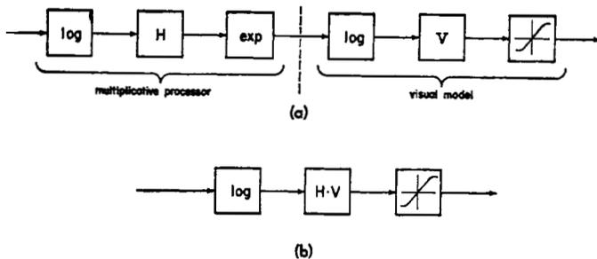
Fig. 12. Total processing system including visual model when viewing Fig. 11(b). (a) Unsimplified system. Processed intensities appear at the vertical dotted line. (b) Simplified system with processors merged.
