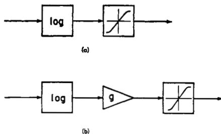
Fig. 13. Total processing system when viewing an image which has been subject to a multiplicative processor the linear component of which has been adjusted to be the inverse of the linear component of the visual model. (a)  $H$  is exactly the inverse of  $V$ . (b)  $H$  is the inverse of  $V$  except for a constant of proportionality  $g$ .
