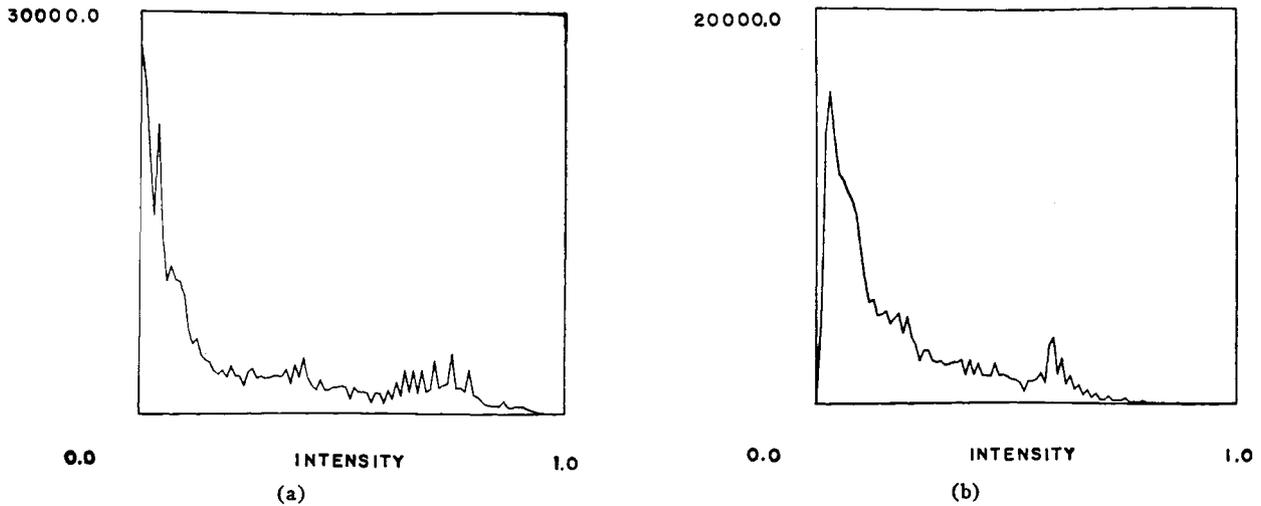
Fig. 4. Intensity histograms of 100 bins each obtained from high quality images carefully digitized to 340 by 340 samples using 12 bit/sample. (a) Three wide dynamic range scenes. (b) Two scenes of less dynamic range (approx. 30:1).
