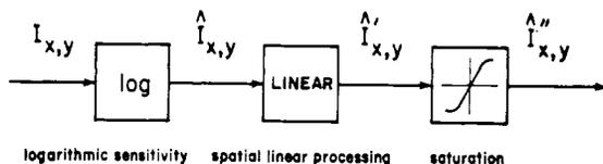
Fig. 10. A possible approximate model for the processing characteristics of early portions of the human visual system.
