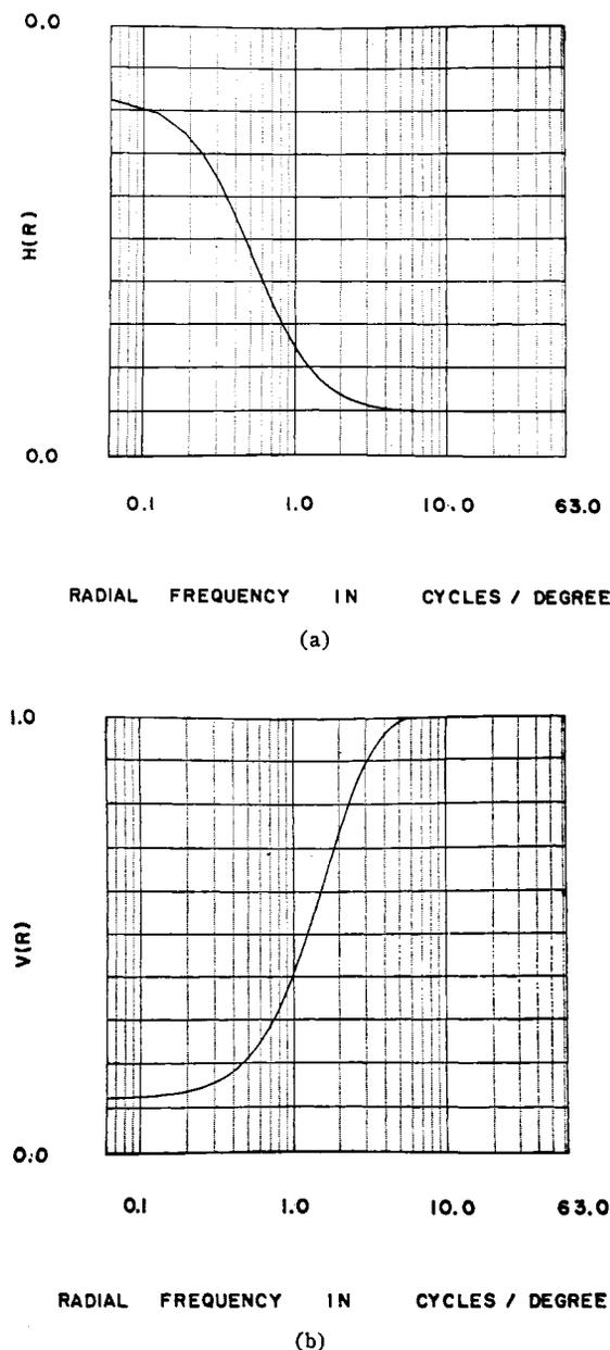
Fig. 16. Frequency response of one-dimensional systems used in test of eye model. (a) Response of system  $H$  for cancelling illusions. (b) Relative response of system  $V$  as estimated from  $H$ .
