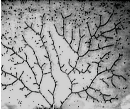
electrorheological fluid with metal spheres
