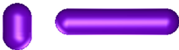
FIG. 11. Three-dimensional spherocylinders composed of a cylinder with length L , capped at both ends with hemispheres with radius R . Left panel: A spherocylinder with aspect ratio L/R = 1 . Right panel: A spherocylinder with aspect ratio L/R = 5 .
