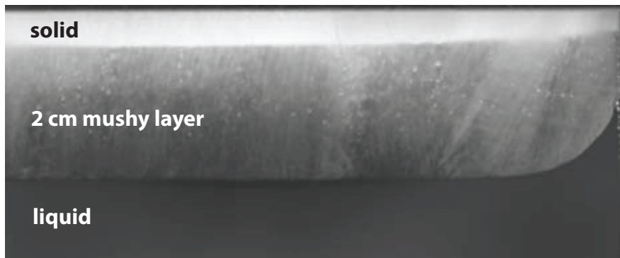
NaCl-H 2 O in lab (Peppin et al., 2007, J. Fluid Mech.)
