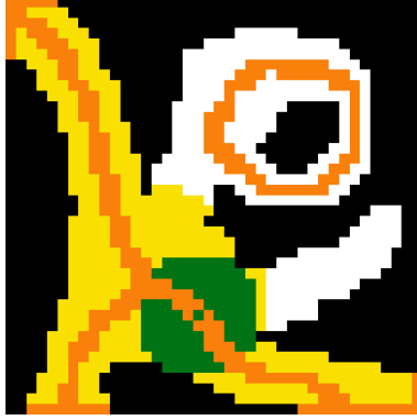
Figure 2.5: The backbone (BB), shown in yellow, is the union of maximal disks centered on the percolating part of the SKkeleton by Influence Zones with boundary (SKIZb), here shown in orange. For the green SKIZb-pixel the maximal disk associated with it is shown.
