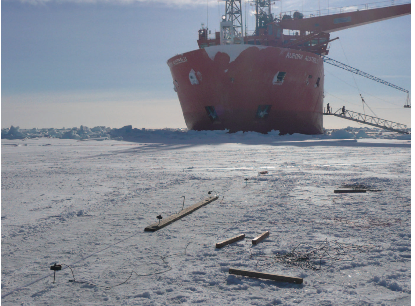
Figure 1: A Wenner electrode array along the surface of Antarctic sea ice, with the Aurora Australis in the background. A current I is injected through the outer electrodes C1 and C2. The potential difference \Delta V resulting from the current flow is measured at the inner electrodes P1 and P2.
