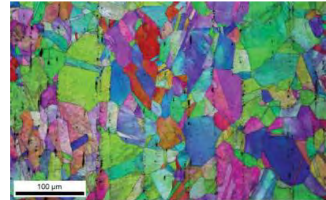
EBSD grain orientation map for copper
