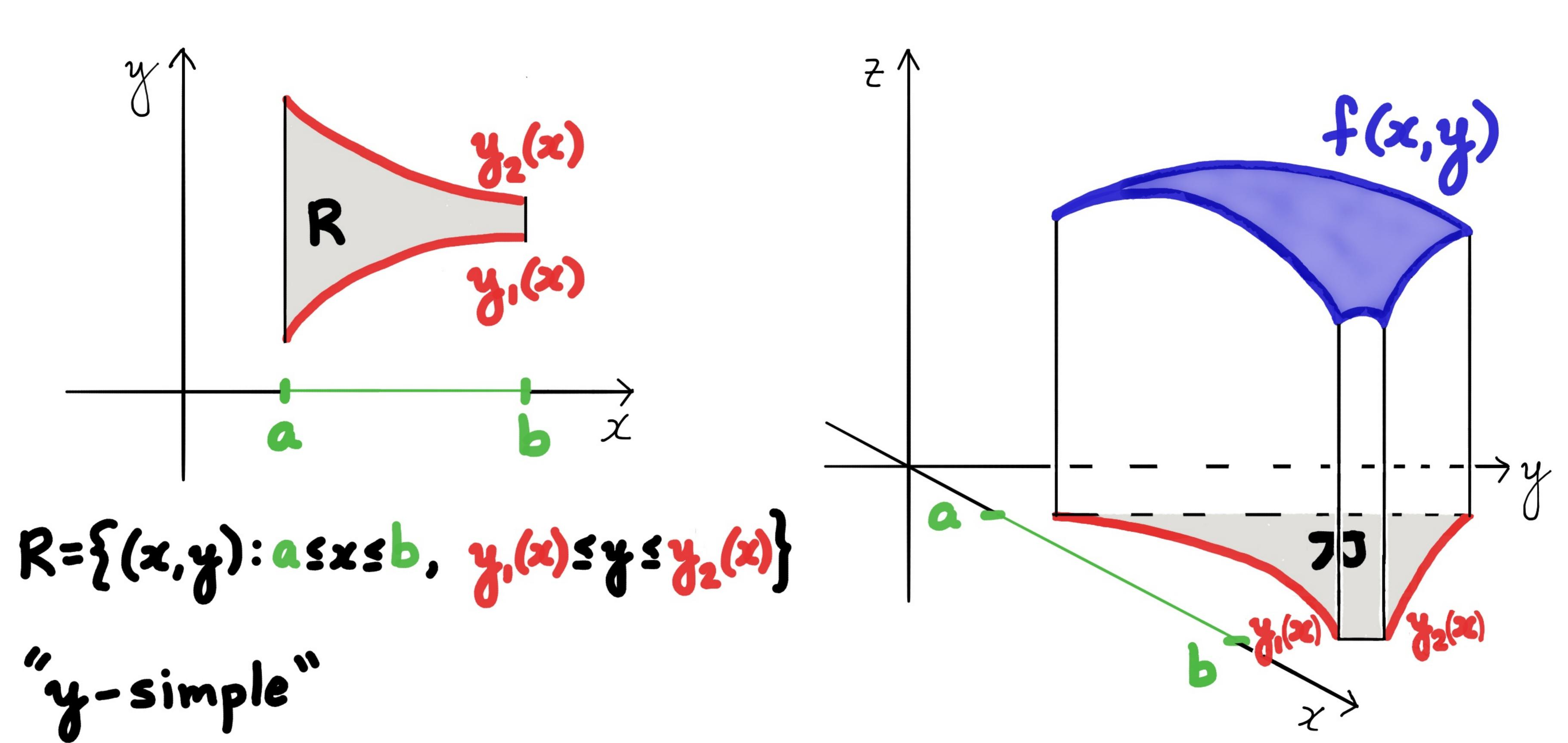
$$\iint_{R} f(x,y) dA = \int_{a}^{b} \int_{y_{1}(x)}^{y_{2}(x)} f(x,y) dy dx$$
