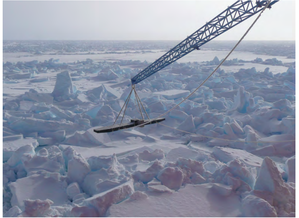
The Worbot - a low frequency EM induction instrument for measuring sea ice thickness
