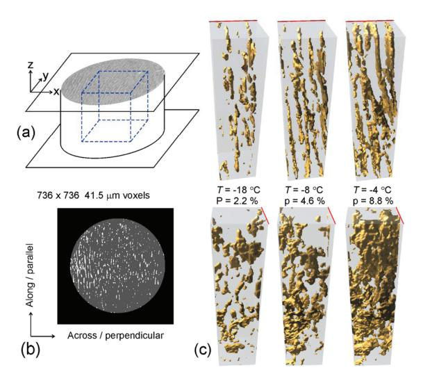
X-ray measurements performed with Skyscan 1074 fan-beam x-ray source micro-CT scanner, in a temperature-controlled sub-chamber of the cold room in which the samples were grown and prepared, returning a 3D image of x-ray absorption.
