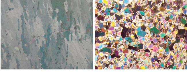
Figure 3: Cross-polarized images of columnar sea ice from the Ross Sea on the left (Langhorne, Golden), and granular ice from the Bellingshausen Sea on the right (Tison).
