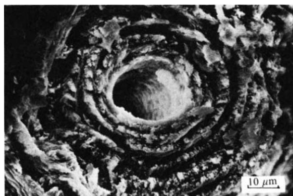
Fig. 2 Fractured surface of a bovine osteon deproteinised with ethylene diamine.
