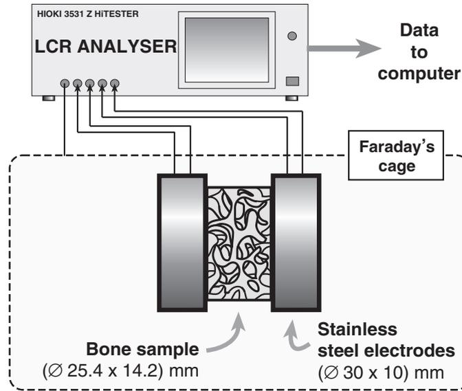
**Figure 1.** Measurement set-up for the determination of bone electrical and dielectric properties. The electrical and dielectric properties were investigated by applying electrical current to samples through two round ( $d = 30$  mm) stainless steel (AISI316L) electrodes using an LCR meter (HIOKI 3531 Z HiTester, Koizumi, Japan). Electrical measurements were conducted in a Faraday cage.
