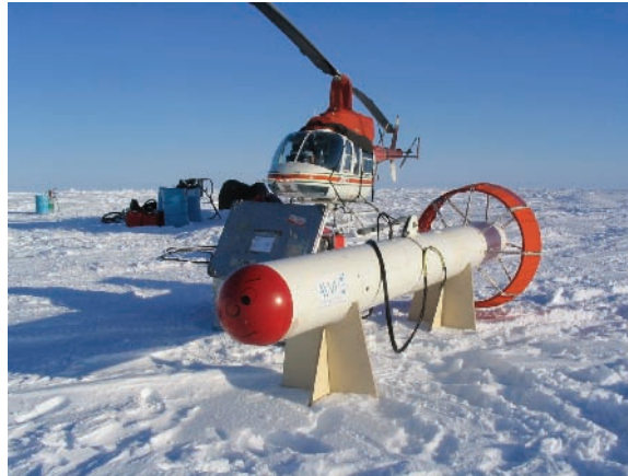
Fig. 4.10 The Alfred Wegener Institute's EM-bird with its towing helicopter in the background on an ice floe in the Arctic (photo by S. Goebell).
