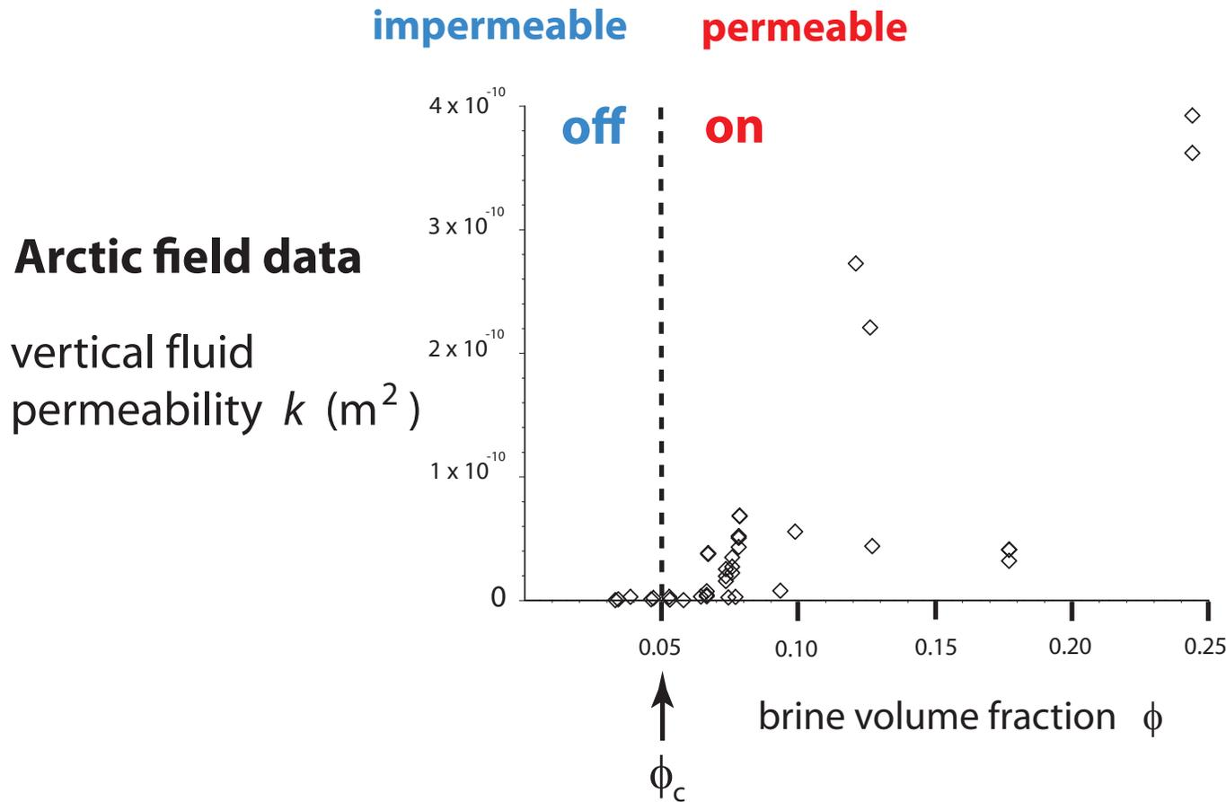
**“on - off” switch for fluid flow**
