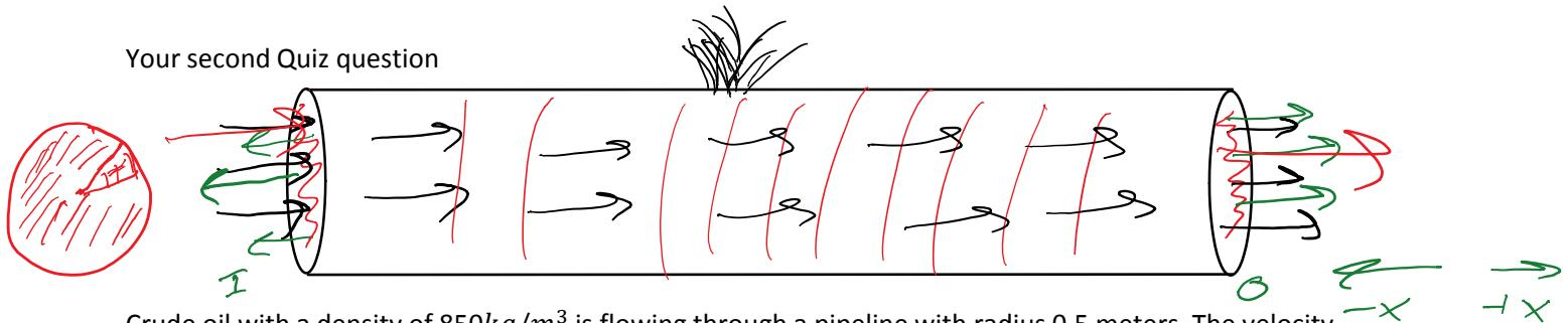
Crude oil with a density of  $850 \text{ kg/m}^3$  is flowing through a pipeline with radius 0.5 meters. The velocity of the oil in the pipe is measured at 2 m/s at the input and remains constant throughout its trip.
