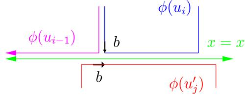
FIGURE 3. Adjacent parallel segment should be viewed as overlapping.
