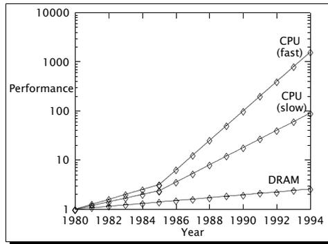
**Figure 1: CPU and memory performance.** This drawing uses 1980 as a baseline. Memory speed (dynamic random-access memory, DRAM) is plotted with an annual 7% increase. The slow CPU line grows at 19% annually until 1985, and at 50% annually since then. The fast CPU line rises at 26% annually until 1985, and at 100% annually since then. The data is taken from [73, Fig. 8.18, p. 427], but extended beyond 1992.
