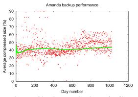
As expected, evolution of hardware technologies for file servers, networks, and tape systems has not had much effect on compression ratios. The worst-case numbers in this plot are highly relevant: they must not exceed tape capacity, since the backup software is not capable of splitting savesets across tape volumes.
