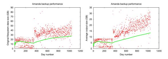
The upgrade, at about day 450, from 8mm Exabyte to DLT 7000 tape is dramatically evident in both these plots: DLT tapes have higher capacity.
