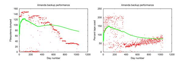
The fall in the number of filesystems beginning about day 500 reflects the upgrade from four Sun SPARC 20/512 fileservers to a single Sun Enterprise 5500 with dual RAID filesystems and larger filesystem partitions.
