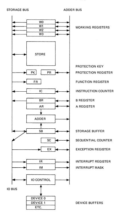
SE, AE, and BE denote extensions of the registers SB, AR, and BR used in floating-point operations.
