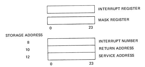
Only the instruction counter is stored as return information about the interrupted program. The interruption program is responsible for saving and restoring the contents of the working registers and the exception register.
