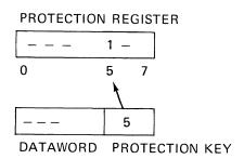
In this system, the monitor can change the protection sphere of a subordinate program immediately by loading the protection register with another bit pattern.
