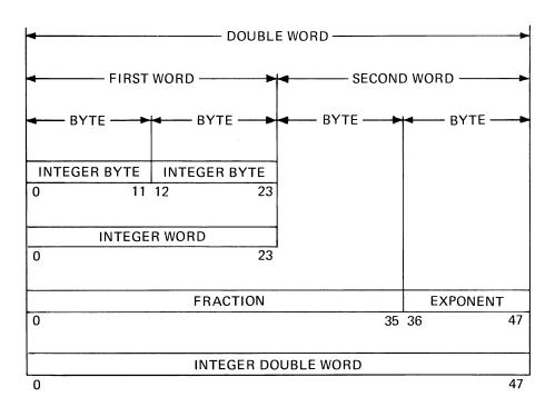
The basic arithmetic operand is an integer of 24 bits. Small integers are packed with two bytes per word. The 12-bit bytes are directly addressable. Double words are used to represent integers of 48 bits and floating-point numbers with 36-bit fractions and 12-bit exponents.
