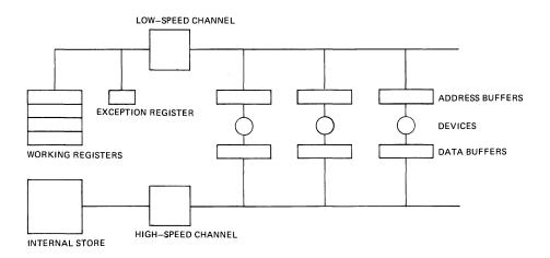
Block transfers can take place on several devices at one time. A multiplexer switches rapidly among the devices connecting them to the high-speed channel, whenever they are ready to transfer a complete data-word to or from the store.
