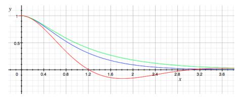
For the same constants, the graphs of solutions beginning with x = 0 and x' = 1 for over/critically/under damped are different colors red/blue/green
