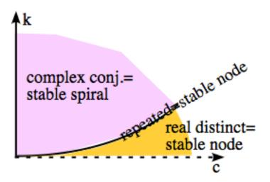
If the roots are complex, the spring system is underdamped and the solution from either condition oscillates infinitely often. If the roots are repeated the system is critically damped. If the roots are real distinct, they are both negative and the system is overdamped. In the critically and overdamped cases, the solution may overshoot x = 0 at most once. However, with the given initial conditions, in these cases the solution returns to x = 0 monotonically.
