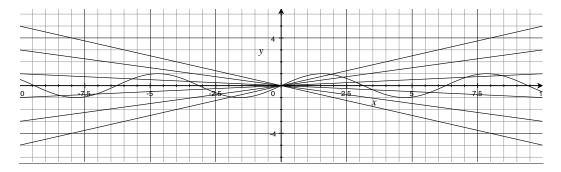
The equations  $y = \sin x$  and y = ax for  $a = \pm .1, \pm .3, \pm .5$  are superimposed. The zeros of  $ax + \sin x$  are the intersection points. So when a = 0 the rest points are at  $\pi k$  for integer k and the flow directions alternate in each interval. As a moves from zero, the line y = -ax intersects  $y = \sin x$  at finitely many and fewer and fewer points. When a = .1 then there are only five rest points. The stable/unstable pairs move toward each other as a increases and vanish.
