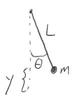
We can apply the conservation of energy to the pendulum to derive the differential equation:
