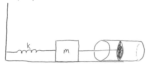
We have a mass on a spring connected to a dashpot. The forces on the mass are:
