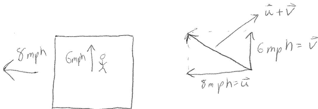
$$|\vec{u} + \vec{v}| = \sqrt{(8 \text{ mph})^2 + (6 \text{ mph})^2} = \sqrt{100 \text{ mph}^2}$$
