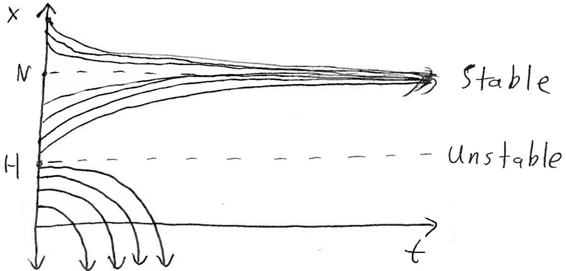
We can see that around  $N$  we have a stable critical point, and around  $H$  we have an unstable critical point. What this means is that for any initial value greater than  $H$  our population size will approach  $N$  as time goes on. For any initial value less than  $H$  our population size will approach  $-\infty$  in a (finite!) amount of time. Of course in reality you can't have less than 0 fish, and so the model would definitely break down when the population becomes sufficiently small.
