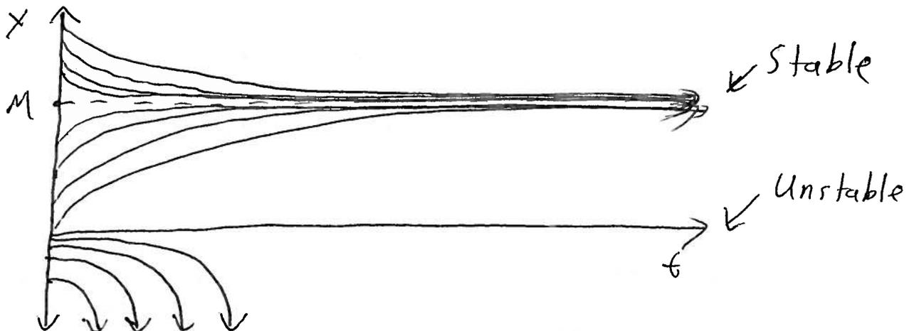
We can see that for the critical point  $x = M$  we have a stable critical point, and that solutions around the point "funnel" towards it. The critical point  $x = 0$  on the other hand is an unstable critical point, and we can see that solutions close to it diverge.
