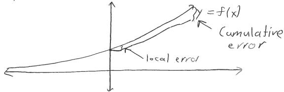
The other source of error is cumulative error. Because in each of our steps we introduce some local error, the starting points from which we calculate the slopes for each step are also not quite right, and so the slopes we calculate are not quite right, and so this introduces even more error. The overall cumulative effect of this error is called, not terribly creatively, cumulative error. It's meant to represent the total error (distance) of our approximate solution from the actual solution.
