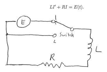
Suppose that L = 5H,  $R = 25\Omega$ , and the source *E* of emf is a battery supplying 100*V* to the circuit. Suppose also that the switch has been in position 1 for a long time, so that a steady current of 4*A* is flowing in the circuit. At time t = 0, the switch is thrown to position 2, so that I(0) = 4 and E = 0 for  $t \ge 0$ . Find I(t).
