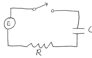
Suppose an emf of voltage  $E(t) = E_0 \cos \omega t$  is applied to the *RC* circuit at time t = 0 (with the switch closed), and Q(0) = 0. Substitute  $Q_{sp}(t) = A \cos \omega t + B \sin \omega t$  in the differential equation to show that the steady periodic charge on the capacitor is
