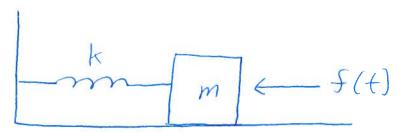
Assuming there is no damping, we can model this system by a differential equation of the form:
