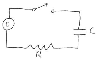
Suppose an emf of voltage  $E(t)=E_0\cos\omega t$  is applied to the RC circuit at time t=0 (with the switch closed), and Q(0)=0. Substitute  $Q_{sp}(t)=A\cos\omega t+B\sin\omega t$  in the differential equation to show that the steady periodic charge on the capacitor is
