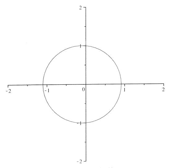
While for Mercury we have a substantially more eccentric orbit: e := .2056
