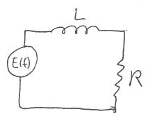
Solution - If we plug the constants L = 2, R = 40, C = 0, and the function  $E(t) = 100e^{-10t}$  into our circuit equation we get:
