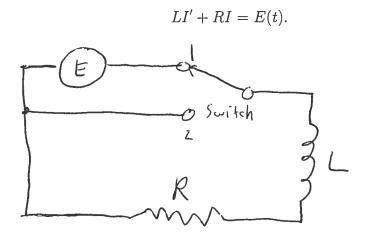
Suppose that L=5H,  $R=25\Omega$ , and the source E of emf is a battery supplying 100V to the circuit. Suppose also that the switch has been in position 1 for a long time, so that a steady current of 4A is flowing in the circuit. At time t=0, the switch is thrown to position 2, so that I(0)=4 and E=0 for  $t\geq 0$ . Find I(t).
