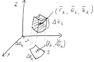
This piece is called a cylindrical wedge, and has volume  $\Delta V_k = \bar{r}_k \Delta z_k \Delta r_k \Delta \theta_k$ . We can approximate the triple integral as:
