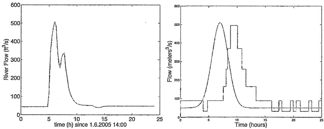
Surge down the Saluda River on 6 January 2005. The solid line is flow at the upstream station and the dotted line is flow at the downstream station.
