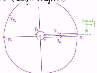
Using a contour like on the previous page wouldn't work for this problem - the real parts of the two key contour integrals *would* cancel out for computing this integral on  $[0, \infty]$ . But the following contour does work:
