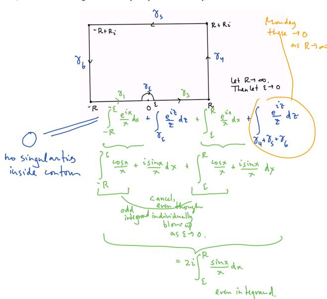
In the previous exercise  $\frac{e^{iz}}{z}$  has a singularity at z = 0 even though  $\frac{\sin(x)}{x}$  is continuous at x = 0.
