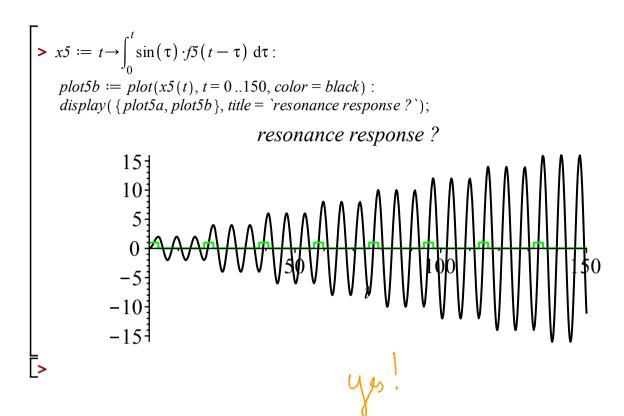
**Hey, what happened????** How do we need to modify our thinking if we force a system with something which is not sinusoidal, in terms of worrying about resonance? In the case that this was modeling a swing (pendulum), how is it getting pushed?
