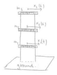
For the unforced (homogeneous) problem, the accelerations of the three massive floors (the top one is the roof) above ground and of mass m, are given by
