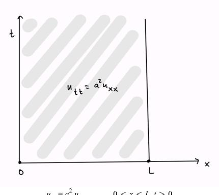
$u_{t\,t} = a^2 u_{x\,x}$  0 < x < L, t > 0u(x, 0) = f(x) initial displacement  $u_{\epsilon}(x,0) = 0$  initial velocity
