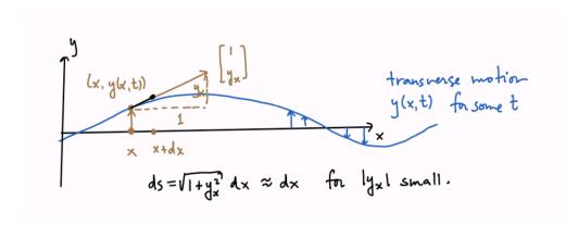
Consider this force diagram. We apply Newton's law to approximate the transverse acceleration of the short segment. The transverse forces arise from the transverse components of the tension-induced forces at the endpoints. Let  $\rho_0$  be the density (mass/length) of the spring.
