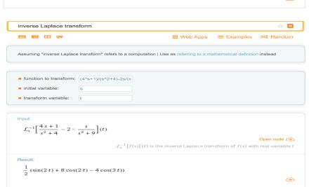
Exercise 6) Use Laplace transform as above, to solve the IVP for the following underdamped, unforced oscillator DE:
