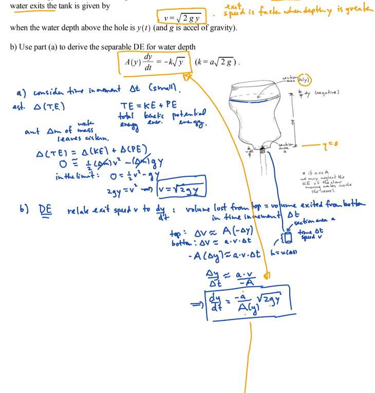
Experiment fun! (We have to postpone this.) I've brought a leaky nalgene canteen so we can test the Toricelli model. For a cylindrical tank of height h as below, the cross-sectional area A(y) is a constant A, so the Toricelli DE and IVP becomes
