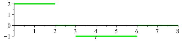
Break the Laplace transform integral from zero to infinity into the sum of integrals over four subintervals (two of the integrals will be zero and use antidifferentiation for the other two), in order to compute the Laplace transform F(s) of f(t).
