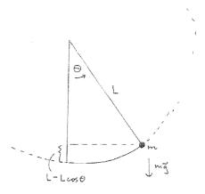
*4a)* Use the fact that the undamped system is conservative, to derive the differential equation for  $\theta(t)$ ,
