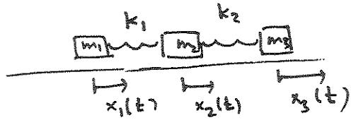
$$\begin{aligned}m_1 x_1'' &= k_1 (x_2 - x_1) \\m_2 x_2'' &= -k_1 (x_2 - x_1) + k_2 (x_3 - x_2) \\m_3 x_3'' &= -k_2 (x_3 - x_2)\end{aligned}$$
