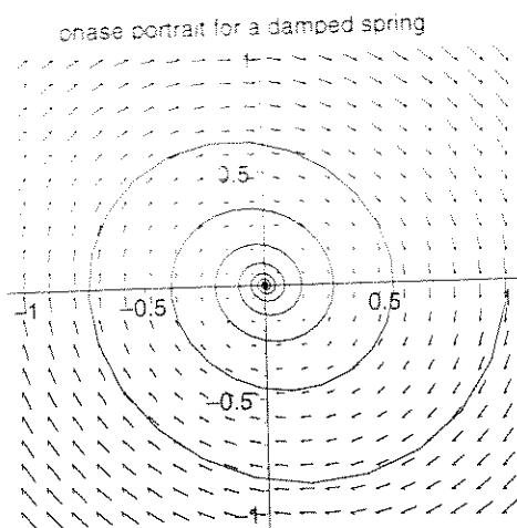
"phase-space picture" for damped mass spring
