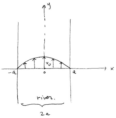
$$v_R(x) = v_0 \left(1 - \frac{x^2}{a^2}\right) \quad \text{river velocity}$$
