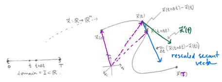
Analytically, the reason that the vector of derivatives  $\underline{x}'(t)$  computed component by component is actually a limit of scaled secant vectors (and therefore a tangent/velocity vector) is:
