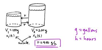
Exercise 1) Find differential equations for solute amounts  $x_1(t)$ ,  $x_2(t)$  above, using input-output modeling. Assume solute concentration is uniform in each tank. If  $x_1(0) = b_1$ ,  $x_2(0) = b_2$ , write down the initial value problem that you expect would have a unique solution.
