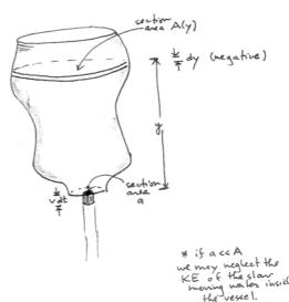
Experiment fun! I've brought a leaky nalgene canteen so we can test the Toricelli model. For a cylindrical tank of height h as below, the cross-sectional area A(y) is a constant A, so the Toricelli DE and IVP becomes
