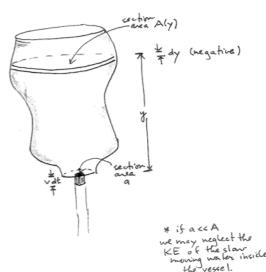
Experiment fun! I've brought a leaky nalgene canteen so we can test the Toricelli model. For a cylindrical tank of height h as below, the cross-sectional area A(y) is a constant A, so the Toricelli DE and IVP becomes
