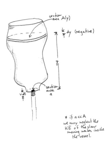
Experiment fun! I've brought a leaky nalgene canteen so we can test the Toricelli model. For a cylindrical tank of height h as below, the cross-sectional area A(y) is a constant A, so the Toricelli DE and IVP becomes
